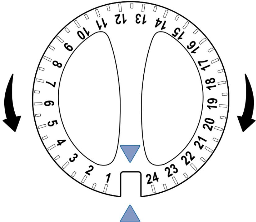
**EN** Replace the battery door and turn the feeder right side up. Open the lids by turning each dial until the arrow on the dial lines up with the arrow on the feeder lid.
