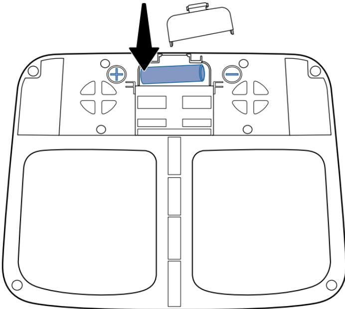
**EN** On the bottom of the feeder, remove the battery door and insert one AA alkaline battery. The battery compartment is very snug—it is easiest to insert the positive (+) end of the battery first, then press the negative (-) end into place.
