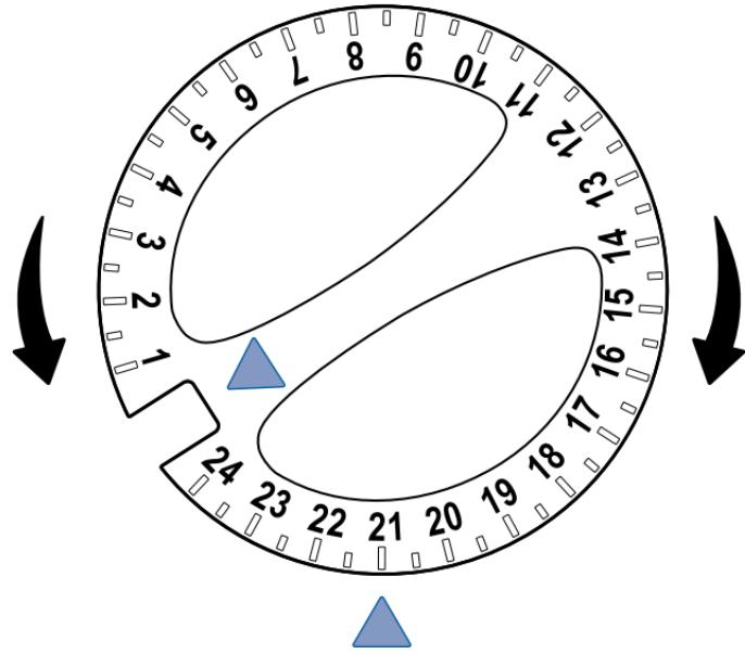
**EN** Set the feeder timers by turning each dial until the arrow on the feeder points to the number of hours between now and when you want your pet to be fed. (You can set it up to 24 hours in advance, in 1/2-hour increments.)
